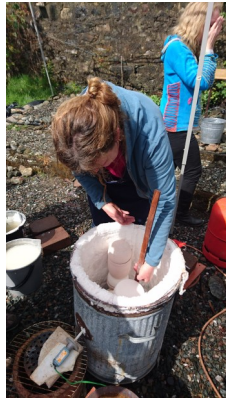
Saggars being packed in a raku kiln.
